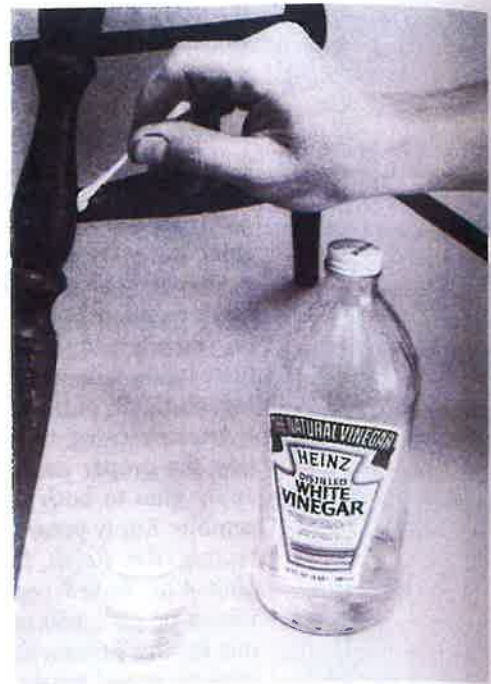
64-5. Use cotton swabs to apply the warm vinegar to joints.
