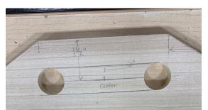
7. Using a jigsaw, cut on the waste side of your line and cut your handle out. Make sure your material is clamped to the table and you are clear from cutting into the table.
