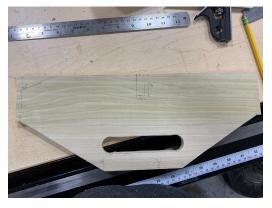
4. On your handle divider mark out your handle. Find the center on the top half of your piece. From the center, mark a line 2" over on either side. Then mark 1-1/2" down from the top edge intersecting both previous lines. These will be your center marks to drill out with a 1" forstner bit.
