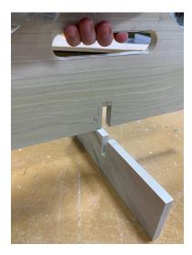
13. To cut your rabbets on either end of your side pieces, mark a <sup>1</sup>/<sub>2</sub>" in from the end of your piece on your edge. Set up your dado blade to <sup>1</sup>/<sub>2</sub>" wide and your sled on the table saw. Set your blade height to <sup>1</sup>/<sub>4</sub>". Use a stop block when setting up your first cut to ensure your next three cuts are identical.
